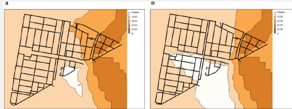
Fig. 7. (a) Pressure's contour before Pressure Management during the critical hour; (b) Pressure's contour after Pressure Management during the critical hour. Pressure in m
